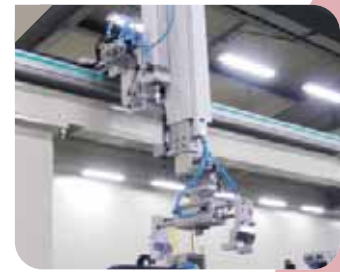
< Core Unloading Unit >
